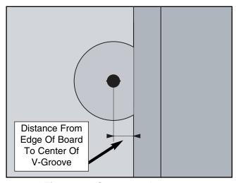
Figure 21. Groove cutting setup. (Top View)
